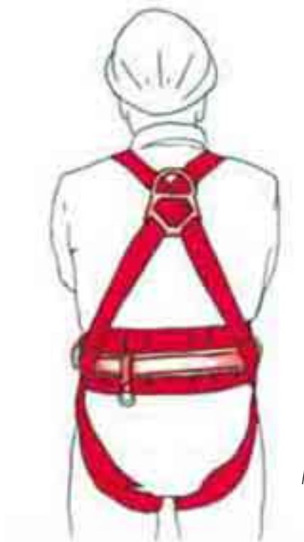
Fig. 14 - Body harness with integrated work positioning belt
