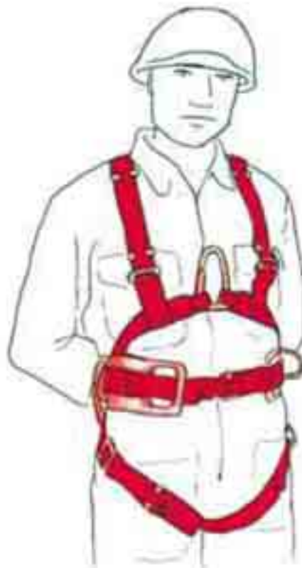
Fig. 15 - Body harness with integrated work positioning belt and sternal attachment
